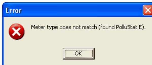
MiniCom 3 successfully performed the meter readout, but the selected meter type doesn't correspond
