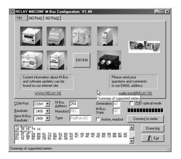
This sheet shows some photos of supported M-Bus devices from the product range of the Relay GmbH, the PadMess GmbH and further manufacturer. Here are also links to the Internet page, from which the current version of the program can be downloaded, and to the email address for criticism and suggestions to the program.
