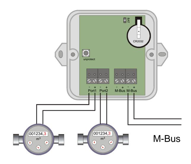
• If not all ports of PadPulse M2 are used, you should not attach a cable to the respective unused port. The capacity of an open-circuited cable reduces the lifetime of the battery in stand-alone operation (no M-Bus available).
