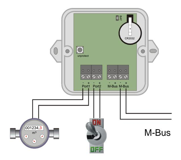
The specifications of the impulse and tariff signal generator can be taken from the technical data. The maximum pulse frequency to be counted is 14Hz.
