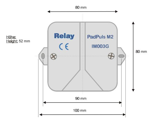
The accompanying drawing defines the measures for wall mounting in mm:
