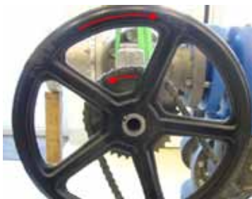
Direction of rotation of hand wheel and chain wheel (chain to be mounted during installation). See step 2 of procedure.
