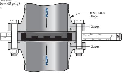
If company policy or jurisdictional regulation requires ASME Code compliance, the rupture disk devices used for pressure vessel overpressure protection shall bear the ASME Code UD symbol. The UD marking is the manufacturer's declaration that the device was manufactured in full compliance with the ASME Code.
