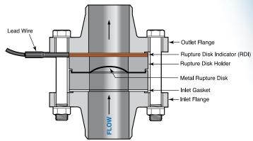
**Note:** RDI is considered a simple device, therefore, approval is not required. Installation must be in accordance with ANSI/ISA RP12.6 and the NEC (ANSI/NFPA 70)
