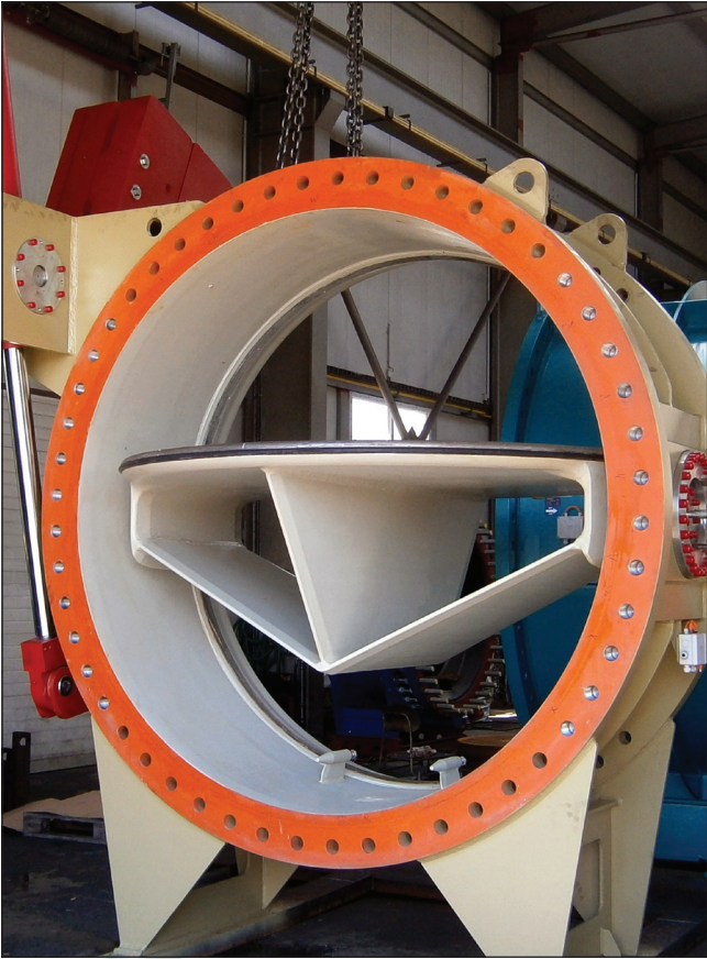
Pic. 10 | Butterfly valve DN2300 PN10 with low-loss disc
