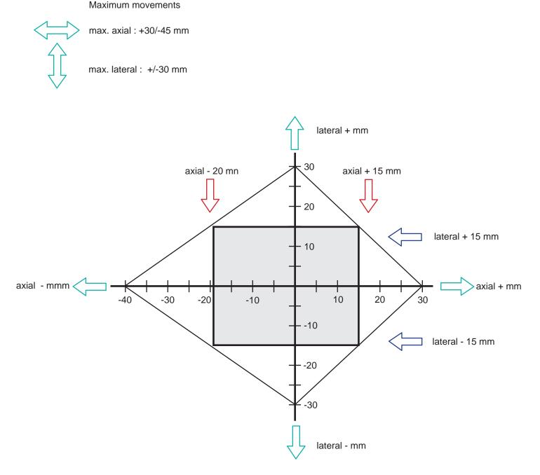
The current movements in combination must fit into the movement diamond as a rectangle.
