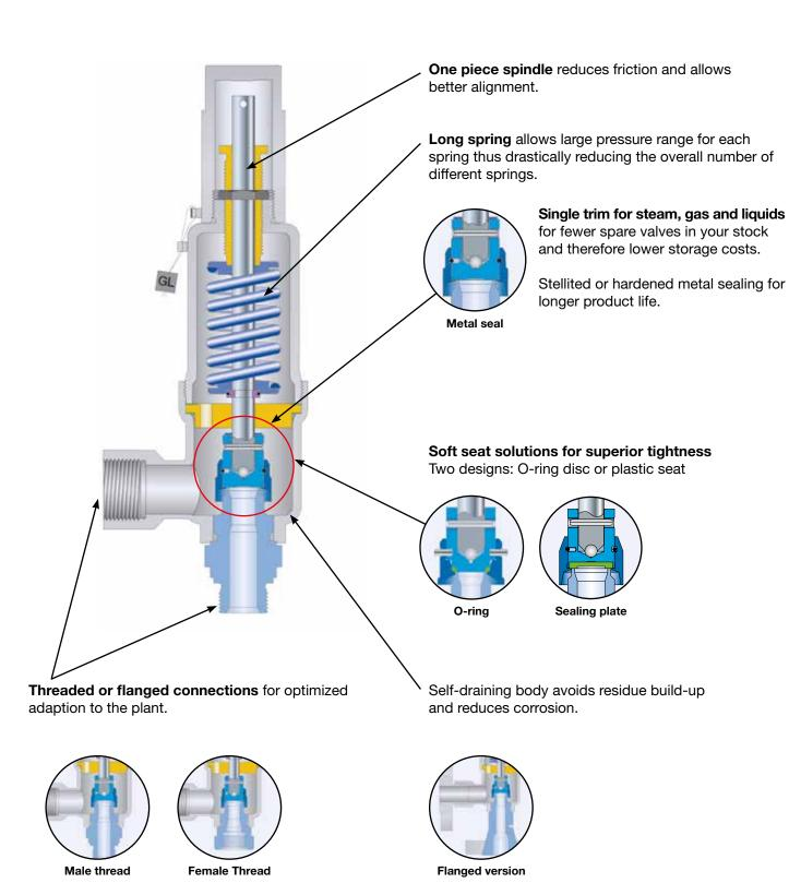
Threaded connections male or female acc. to NPT ANSI/ASME B1.20.1. Threads according to other standards, e.g. ISO, DIN, BSP are also available.
