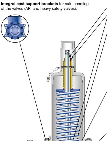
One piece spindle allows better alignment.
